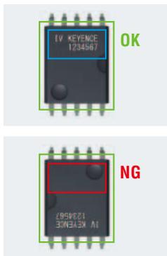
**Detects the direction of the IC in carrier tape**
