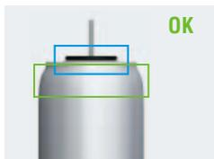
Detects the presence of an O-ring in a spray can
