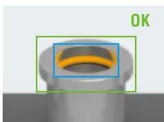
Detects the presence of packing in metallic parts
