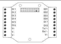
DIx. Discrete IN x DOx. Discrete OUT x
