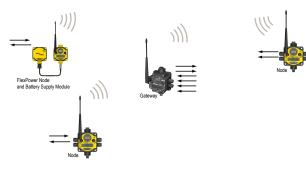
The SureCross® DX80 wireless I/O network provides reliable monitoring without wiring or conduit installation. The SureCross wireless network operates independently or in conjunction with a host system, PLC, and/or PC software.
