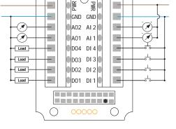
DOx. Discrete OUT x. GND. Ground/dc common connection. PWR. Power, 10 to 30V dc power connection.
