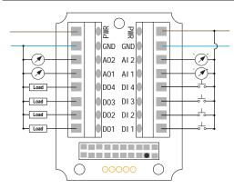
Alx or Ax. Analog IN x. AOx. Analog OUT x. DIx. Discrete IN x.
