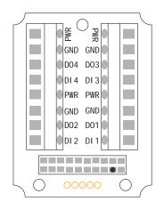
DIx. Discrete IN x. DOx. Discrete OUT x. GND. Ground/dc common connection. PWR. Power, 10 to 30V dc power connection.
