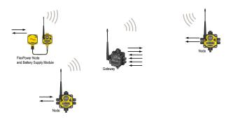
The SureCross® DX80 wireless I/O network provides reliable monitoring without wiring or conduit installation. The SureCross wireless network operates independently or in conjunction with a host system, PLC, and/or PC software.
