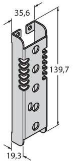
Mounting bracket, for PVA100, coldrolled steel, no cut-out for DIP switch block , protection for light
