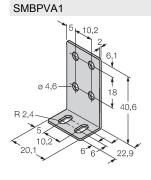
Mounting bracket, for PVA and PVD, stainless steel; set consisting of two brackets and screws
